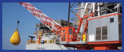
ALATAS supply water bags and load cells for both dynamic and static load tests for Marine Offshore & landbased cranes. ALATAS crane load tests are performed as per **ALATAS** designed protocols, matching individual crane models set out by the manufactures. A certificate is issued upon successful completion.
